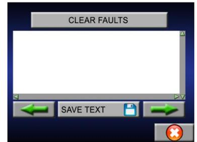
The fault codes can also be saved in a txt. file format to an inserted SD-Card for viewing via a PC/laptop.
