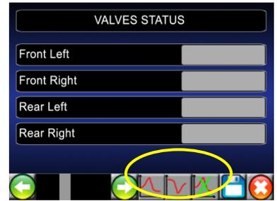
This function is very useful when doing comparison work after making changes or repairs to a system, as well as diagnosing faults.
