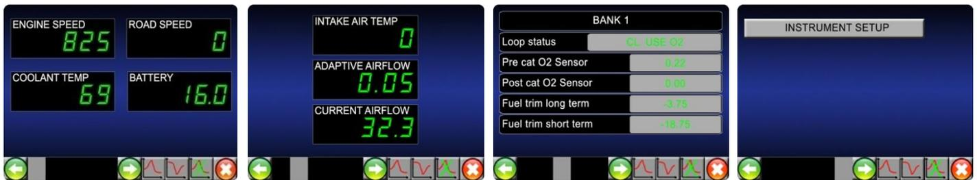
There are several pages of live data inputs for each engine type. The instrument mode is also home to the “peak detection function”. The most common use for the instrument mode is to mount the Nanocom on the dashboard of a vehicle and being able to monitor key engine inputs while the vehicle has its engine running or while in motion, here is the NCOM30 dash-mounting kit that we can supply...
