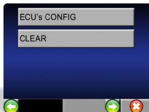
The first three functions simply read the **tested**, **not tested** or **permanent** fault codes, depending on selection, from the vehicle system ECU's that are selected in the **ECU's CONFIG** option. All of these functions will then produce a list of Faults and their definitions in plain text, that can be scrolled through one fault per screen.
