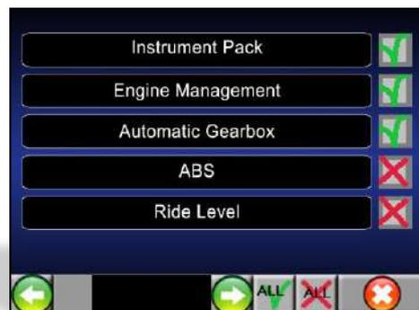
The **ECU's Config** sub-function provides a list of all of the vehicle system ECU's fitted to the currently connected vehicle. This allows for the selection and de-selection of any ECU that the first four fault reading functions will read the fault codes for.
