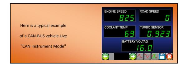
This mode has been created primarily for use while driving the vehicle to observer various data that the vehicle may not display, such as live Mass Air Flow (MAF) into the engine. This can be useful in fault diagnosis or purely as a secondary drivers display.
