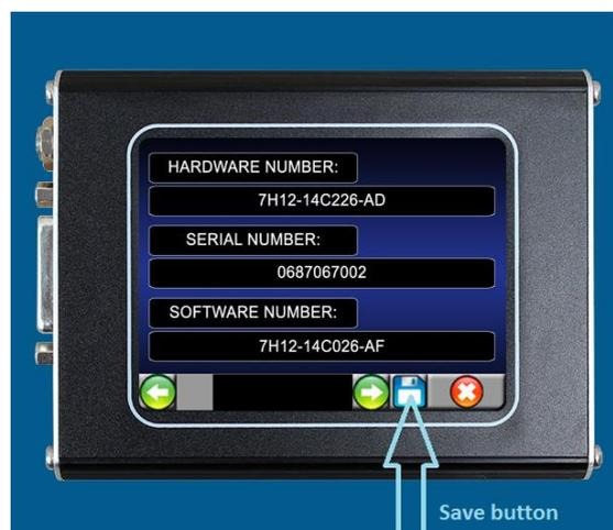
The module information will be saved on the SD Card root as a .txt file. Always back-up the saved modules from the SD Card before starting the Flashing procedure. SD Cards are corruptible resulting in the loss of the initial information containing the modules numbers.
