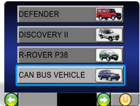
**!** IMPORTANT: Unlike traditional multi-model vehicle diagnostic equipment, for CANBUS vehicles, the Nanocom has NO vehicle model or ECU menus to select from, instead, under the CANBUS VEHICLE option, the Nanocom initiates a "VIN detection" function, which tells the unit exactly which vehicle is currently connected. After the VIN detection process, there is a list of diagnostic and service functions. These are currently (V1.24 onwards):
