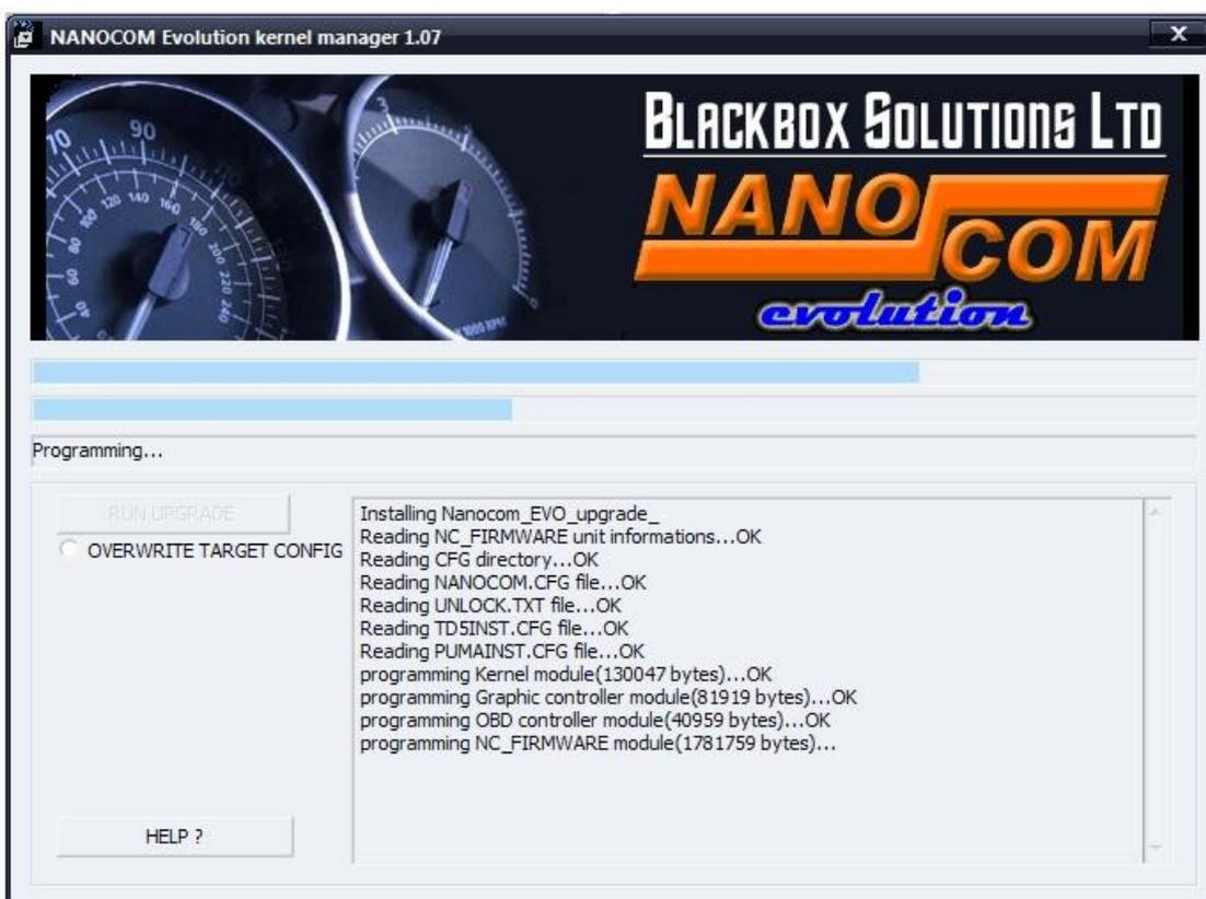
2.6. When the "Upgrade completed successfully " message appears press OK.
