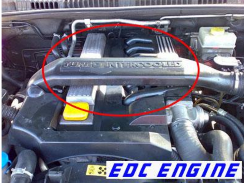
EDC Diesel Engine Management System, Easily identified by the intake tube with the words "TURBO INTERCOOLED" embossed on it.
