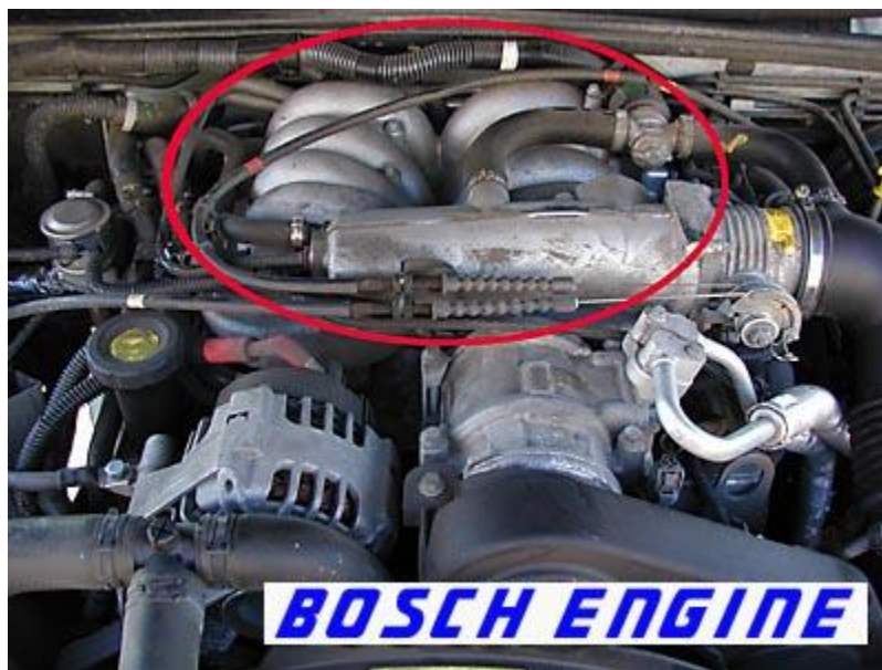
Bosch Motronic Petrol Engine Management System, Identified by it's collection of Banana shaped manifold tubes.
